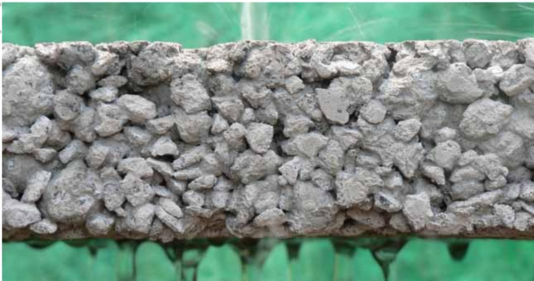
*PerVIOUS pavement allows water from precipitation to pass directly through, thereby reducing the runoff from a site and allowing groundwater recharge.*
